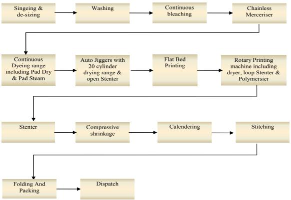
The manufacturing process as shown in the above diagram is explained below:-
